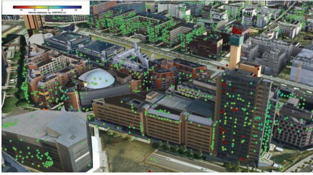
Figure 5. Deformation at the Debris-Tower, visualized using Google Earth
