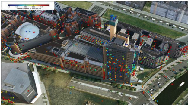
Figure 6. Temporal coherence of the PS points, visualized using Google Earth
