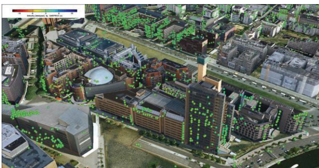
Figure 7. Deformation after filtering at the Debris-tower, visualized using Google Earth
