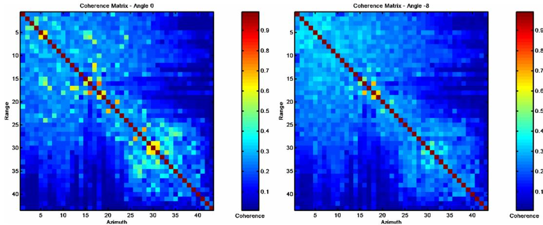
Figure 9. Coherence matrices ordered with respect to temporal baselines. Left: calculated on a linear window along the railway. Right: CEW oriented in a different direction.
