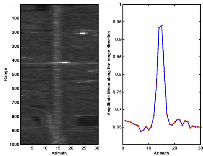
Figure 6. Left: resampled Track 3 reflective map (detail). Right: amplitude mean along the range direction
