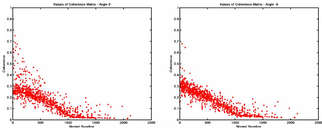
Figure 10. Coherence matrices values of Fig. 9 ordered with respect to normal baselines.
