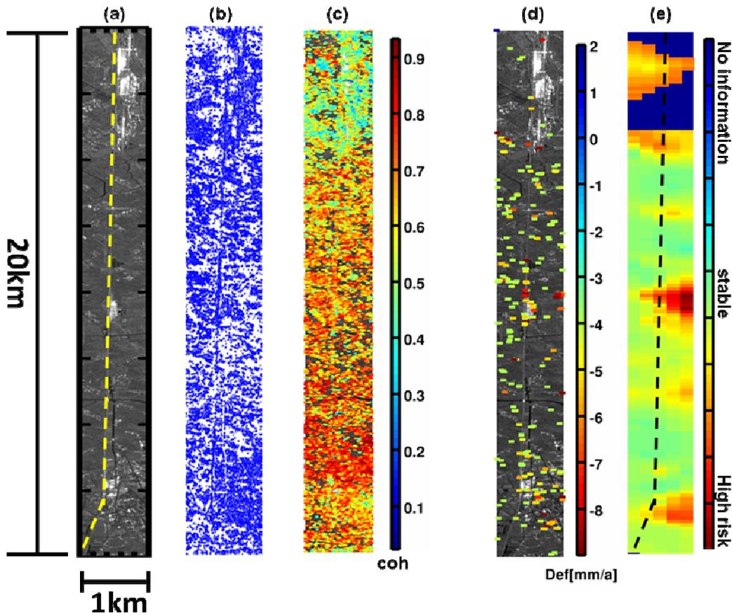
Figure 7. QPS processing results. (a) reflective map, (b) QPS candidates, (c) temporal coherence, (d) QPS with high subsidence trends (e) Kriging interpolated deformation fields, the red areas indicate high risk subsidence regions along the railway.
