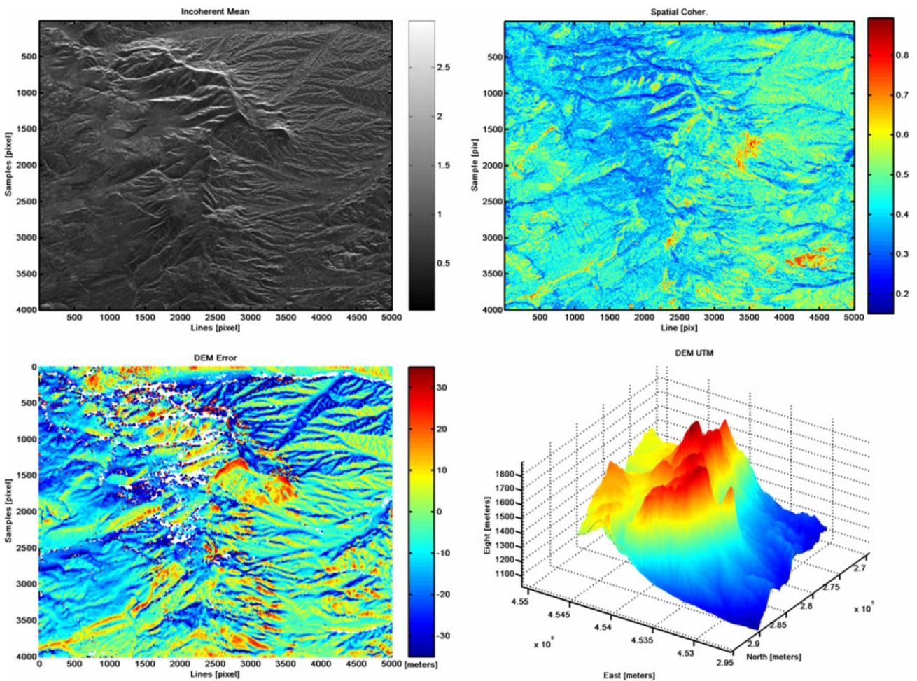
Figure 1. QPS processing results in the mountainous area around the city of Zhangbei. Top left: Incoherent mean of the dataset. Top right: averaged spatial coherence. Bottom left: height error in respect to the SRTM DEM. Bottom right: geocoded DEM (UTM coordinates)
