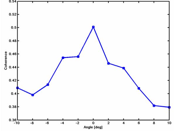
Figure 8. Mean coherence estimates with different angles. The highest coherence estimate is obtained along the railway.
