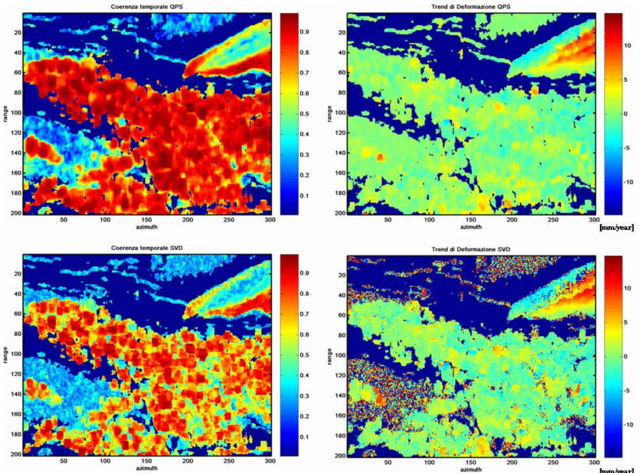
Figure 3. Time series analysis results on a small area next to the Three Gorges Dam. Top left panel: temporal coherence of the QPS analysis. Top right: deformation trends estimated by QPS technique. Bottom left panel: temporal coherence of the SVD analysis. Bottom right: deformation trends estimated by SVD technique.
