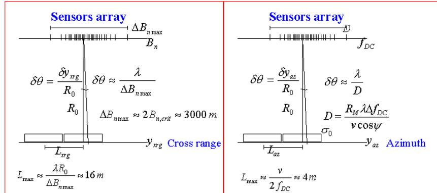
Figure 5: Acquisition geometry referred to the master image.
