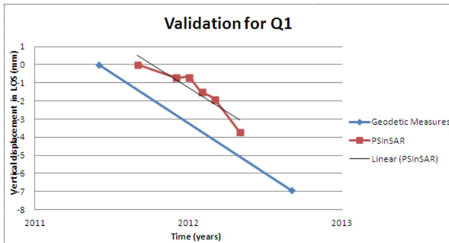
Figure 4: Displacement time-series for Q1 acquired with geodetic and PSInSAR techniques.
