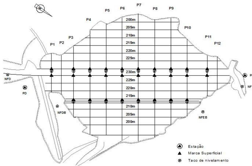
Figure 2: Location of the points from the geodetic network in the Álamos I dam.
