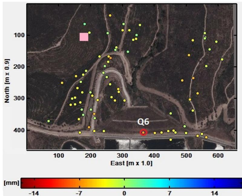
Figure 5: Cumulative displacement for permanent scatterers in Álamos II.
