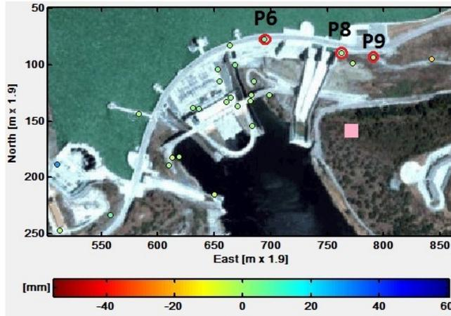
Figure 6: Cumulative displacement for permanent scatterers in Alqueva.
