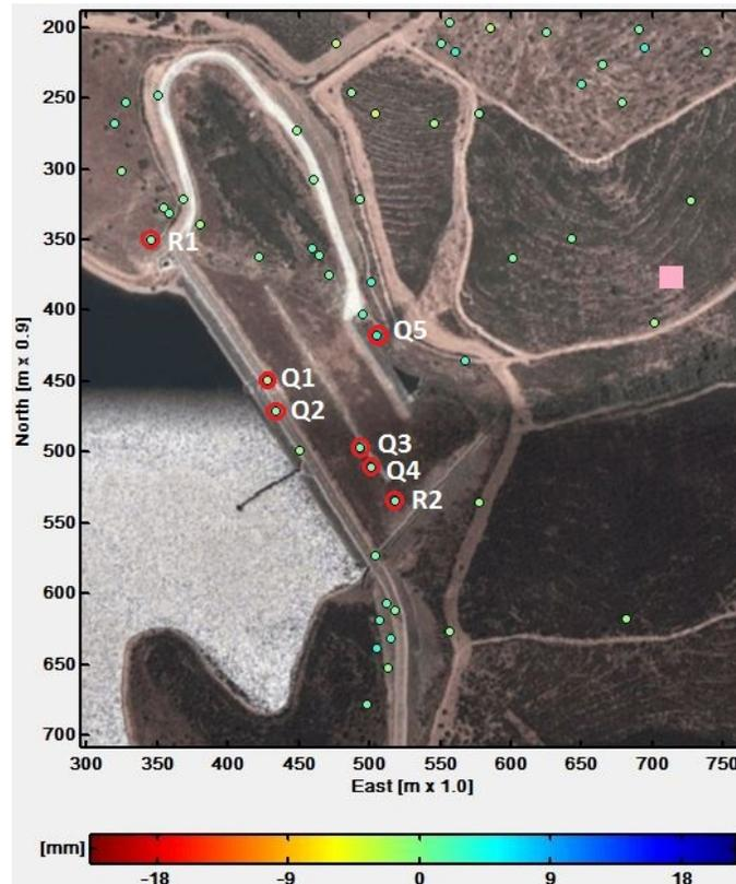
Figure 3: Cumulative displacement for permanent scatterers in Álamos I.
