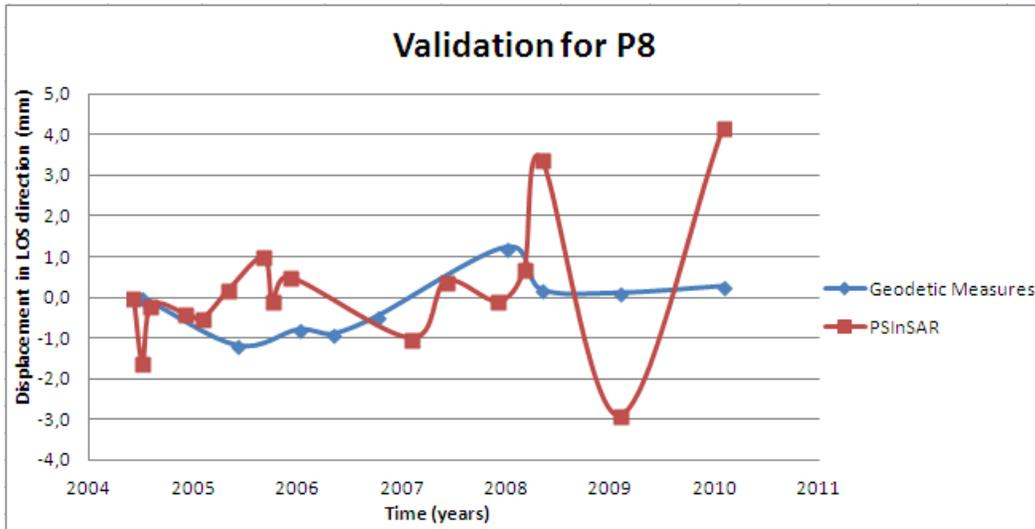
Figure 7: Displacement time-series for P8 acquired with geodetic and PSInSAR techniques.
