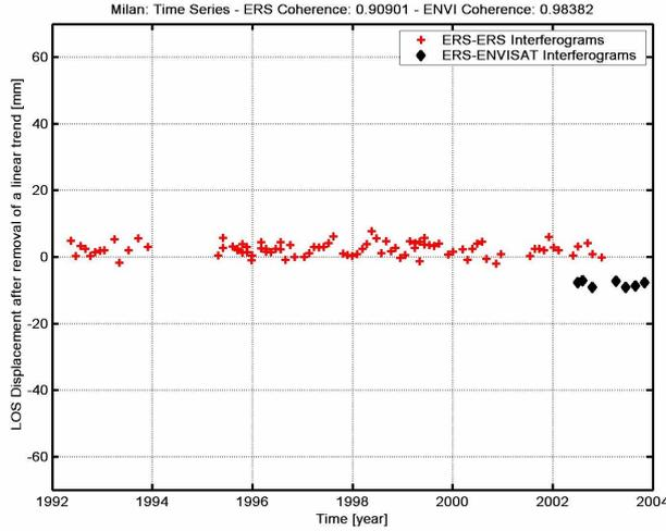
Figure 1. PS time series. ERS-ERS interferograms (red points) and ERS-ENVISAT interferograms (black points).
