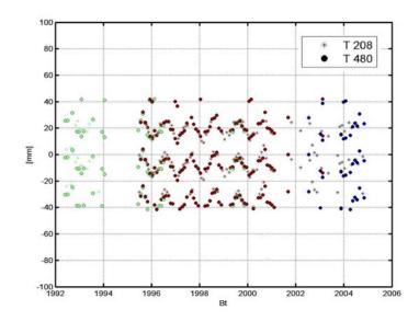
Figure 4. An example of Displacement time series [mm] measured by ERS and ENVISAT from 2 different parallel tracks 40km apart. Stars: track 208, circles: track 480. Green dots: ERS-1. Red dots: ERS-2. Blue dots: ENVISAT.
