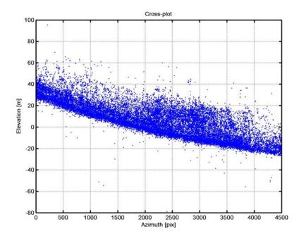
Figure 1. PS's Elevation [m] along azimuth [pixel], which corresponds approximately to the North (left) - South (right) direction.
