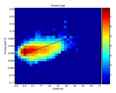
Figure 7. Correlation between PS's thermal dilation [rad/°C] and their elevation [m]. Black line: composite steel concrete building expected trend of thermal dilation as a function of elevation.
