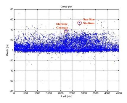
Figure 2. PS's Elevation [m] along azimuth [pixel], after topography removal.
