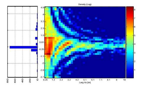
Figure 3. PS's azimuth geometric conformation (Milan dataset). Color scale indicates the density of PS's in a log scale. Y-axis: PS's orientation as a function of normalized Doppler Centroid [Hz/PRF]. X-axis: PS's azimuth extension [m]. This extension can be larger than one cell, as the phase response has central symmetry and the amplitude one is windowed by the ground reflectivity pattern. Left: normalized Doppler Centroids histogram.
