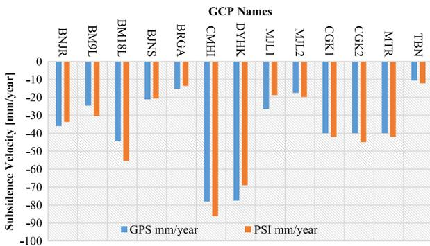
Fig. 6. PSI and GPS confirmation (subsidence velocity).
