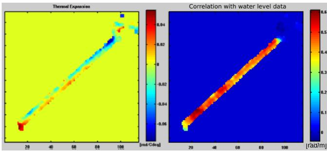
Figure 7. Estimated linear correlation between PSI phase values and temperature (left) and reservoir water level data (right).
