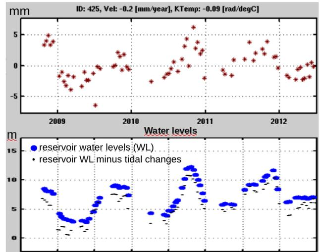
Figure 6. Phase residuals recomputed as deformation in LOS [mm] of selected point on the dam surface (upper figure) and water level of the reservoir [m] during acquisitions (lower figure).
