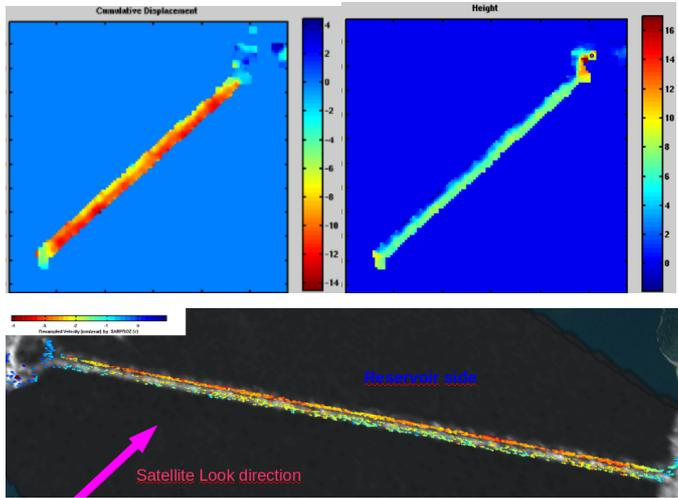
Figure 4. PSI processing result; left: Estimated cumulative deformation of dam (2008-2012 in the satellite LOS), right: estimated height, lower: average rate of displacement geocoded and superimposed over amplitude image.
