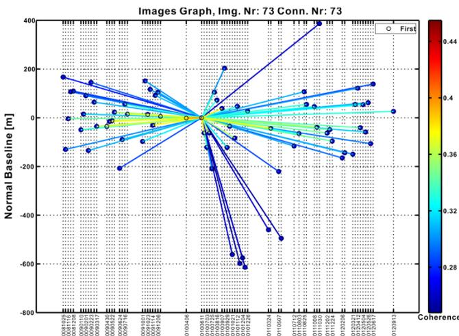
Figure 2. Dataset of TerraSAR-X and TanDEM-X used in the processing: x-axis indicates the temporal baseline and y-axis indicates the normal baseline.
