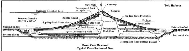
Figure 1. Cross Section of Plover Cove Dam [4]
