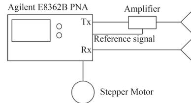
**Fig. 1.** Schematic of the radar system
