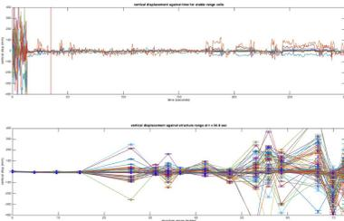
c) Displacement against position along bridge at different time
