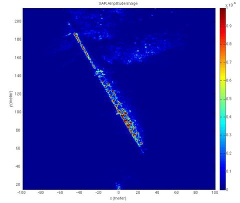
a) Amplitude of the return signal of the bridge
