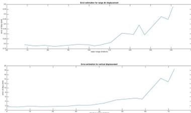
d) Error of range (upper) and vertical (lower) displacement against range
