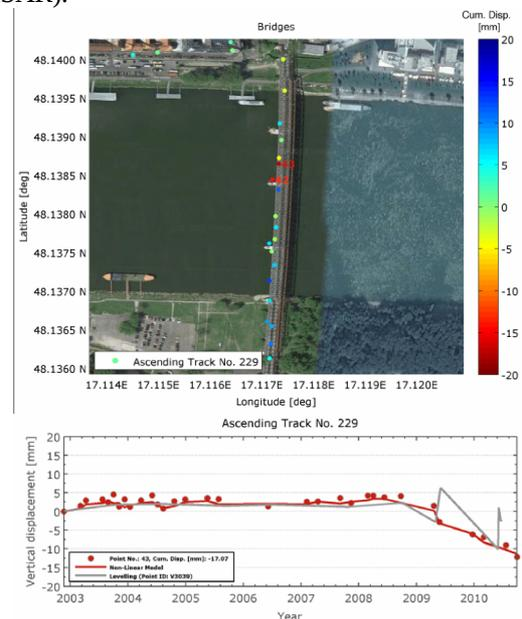
Fig. 1. Levelling vs. PSInSAR time series over bridge that was affected by the crash of a tug in 2010.
