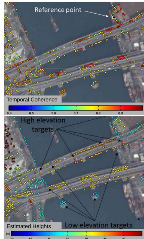
Fig. 4. Temporal coherence (a) and estimated heights (b) of Cheung Tsing bridge analysis.
