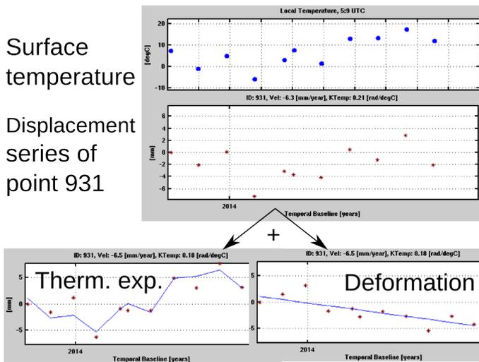
Fig. 3. Decomposition of displacement series of point 931 into thermal expansion and temporal deformation components. Potential errors are caused by inappropriate dataset (at least two year cycles are needed).
