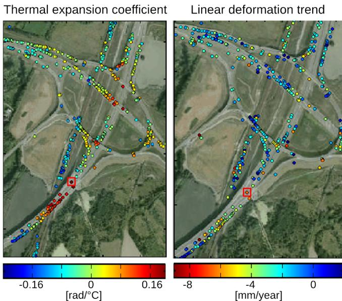
Fig. 2. Thermal expansion coefficient and linear deformation trend values of Ostrava-Svinov roundabout estimated using 11 TerraSAR-X Stripmap images (2013-2014). Red square depicts selected point 931.
