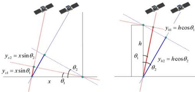
Figure 4. Misregistration between two parallel tracks due to a different height.
