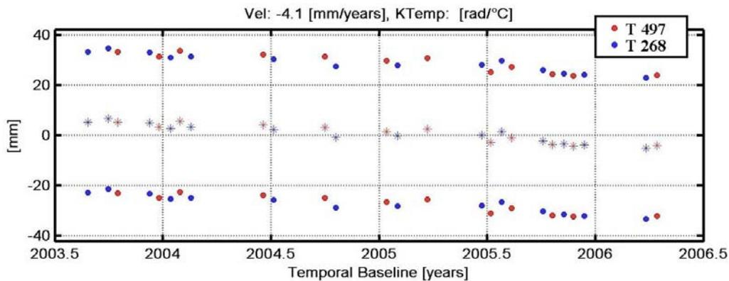
Figure 6. Displacement time series of a PS detected in Shanghai as estimated from the joint combination of two Envisat parallel tracks (T497 red dots, T268 blue dots). The two adjacent replica are plotted for visualization purposes. The combination of parallel tracks allows halving the revisit time.
