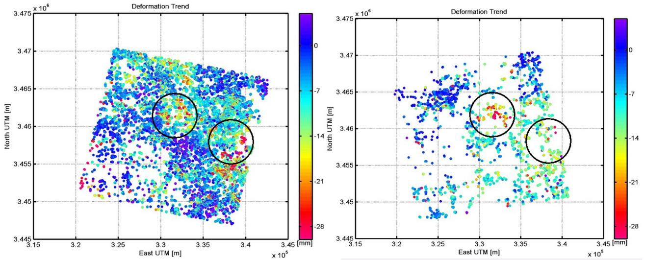
Figure 5. PS velocity fields in Shanghai estimated from an ERS descending track (left, ~30000 PS's) and from the joint combination of two Envisat ascending tracks (right ~5000 PS's). The two black circles highlight the subsiding areas detected in both analysis.
