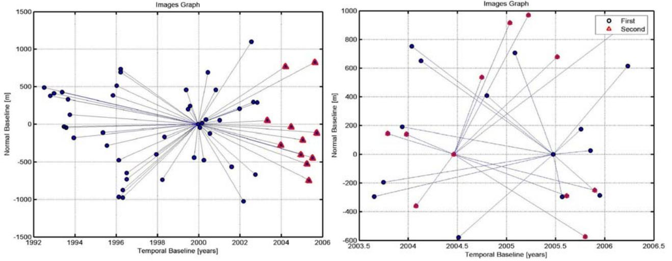
Figure 3. Different strategies to exploit ASAR data. Left: coherent combination of ERS (blue dots) and Envisat (red triangles) data of the same track, in a single master configuration. Right: uncoherent combination of parallel tracks, in a double master configuration. The two plots represent the images in the normal-temporal baselines space. Data are relative to the Shanghai test site (left Track 3, right Track 268 and 497).
