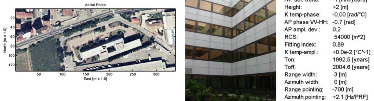
Fig. 10. PS example in Milan: trihedral in a court-yard. Left: aerial photo and PS position. Centre: target photo. Right: list of the PS estimated parameters (height h=2m , high RCS, small L_x=3m L_y=0m , AP phase -0.7rad ).
