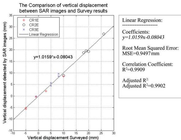
Figure 6. A statistical analyses on the deviation between the displacement detected by InSAR and by optical leveling measurement.
