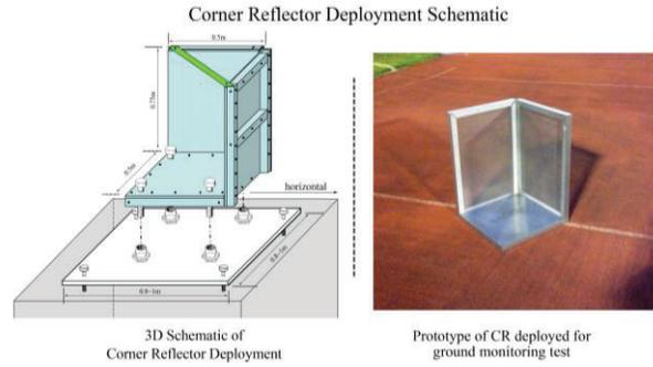
Figure 2. Schematic of Corner Reflector deployment.
