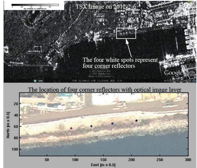
Figure 3 Upper: the location and intensity of the four CRs on TSX images. From the image we can see that the background radiation in that area is very low, and the intensity of CRs is considerably high. Down: the location of CRs geocoded to optical image. The location is near the sea that is identical for its low intensity in RADAR images.
