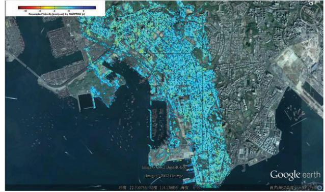
Figure 4. Linear Displacement Map for PSs that have a height within the region of [-5,5] meters.
