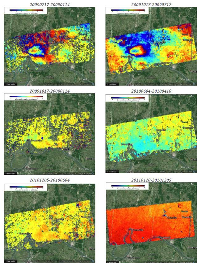
**Fig. 2.** Interferograms between L-band ALOS image pairs
