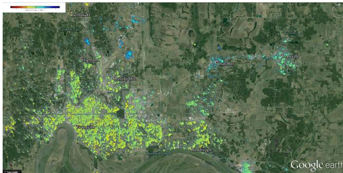
**Fig. 6.** The velocity map of PSI analysis using ERS C band data stack
