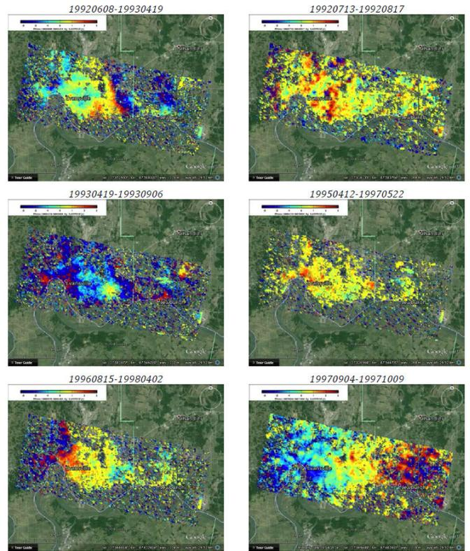
**Fig. 4.** Interferograms between C-Band ERS1&2 image pairs
